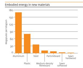
**Note:** The value for plastic is for PVC (polyvinylchloride). The values for timber are for kiln-dried timber.
