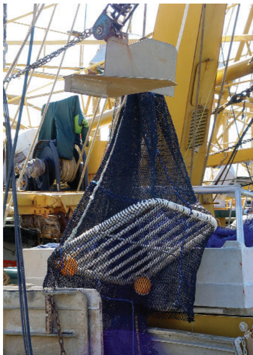
TED fitted to trawl net
